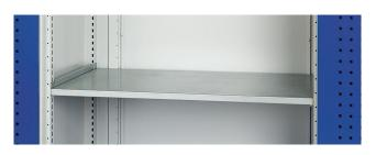
Durable, scuff resistant galvanised steel shelves, 100kg U.D.L. capacity. Adjustable on 25mm pitch.
