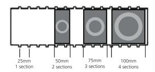
Any combination of CNC inserts may be used together in a single row up to the maximum number of sections per row.
